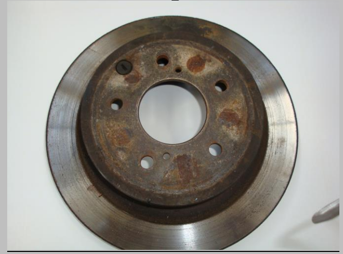
Rotor outer bearing interface
